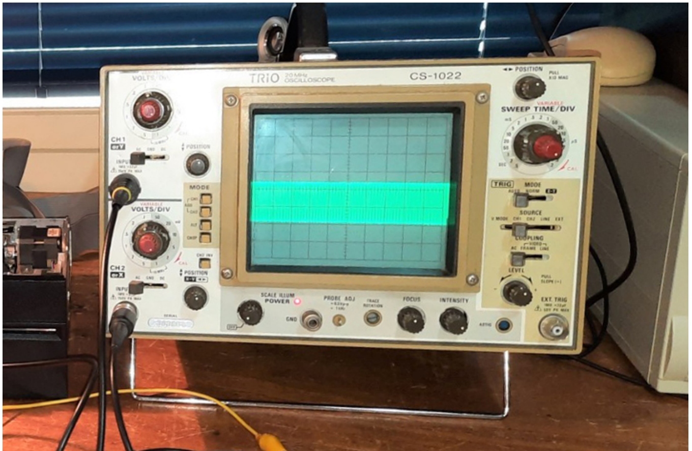
Figure 7. A strong signal after "coarse tuning" with the stepper coupling (note: each division in this case is 100mv)
