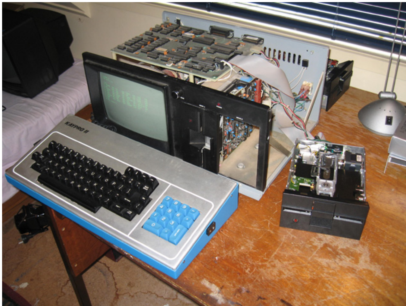
Photo 1. Kaypro hooked up to another one of my full-height drives to verify the disk controller was ok.
